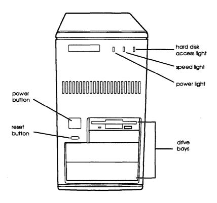
The power indicator lights up. After a few seconds, the computer performs its power-on diagnostics. This is a series of checks the computer runs each time you turn it on to make sure everything is working correctly.
